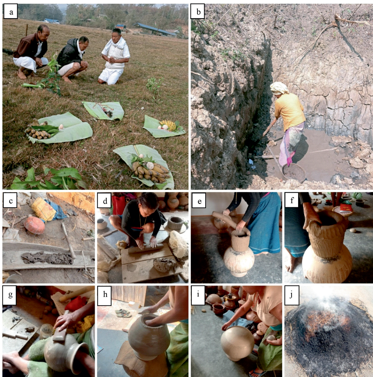
Figure 6: Images showing Andro pottery manufacturing process (a)-Leibak Leithong Hangba ceremony, (b)-raw material collection, (c)- pounded raw materials, (d,e,f)- rolling and joining circular strips, (g)- beating, (h)-Base formation, (i)- polishing (j)- firing. (Photo credit: Authors)
